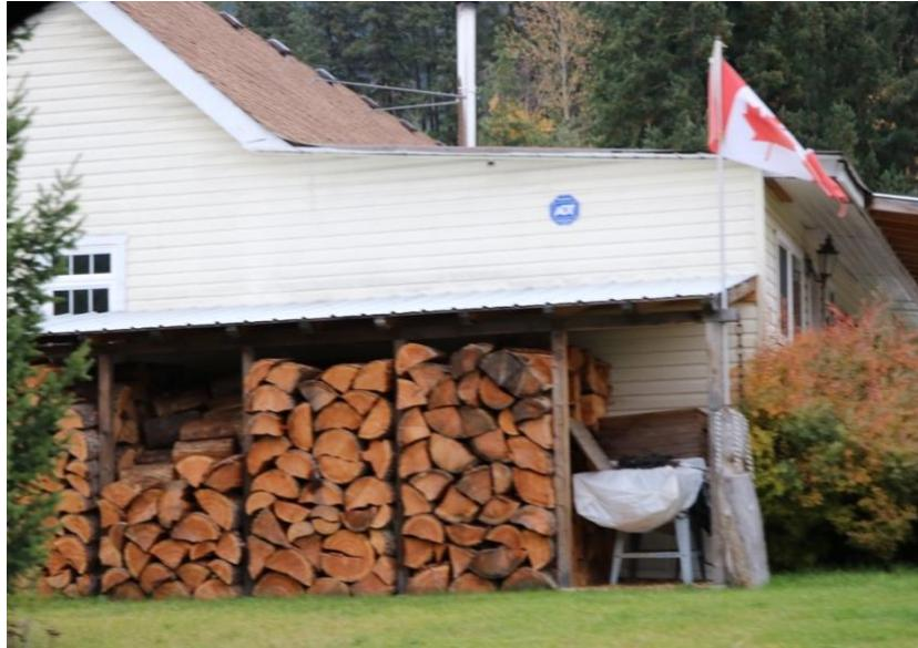
*Figure 10 Ignition of outbuildings with 15m of a home pose a significant risk to home ignition due to prolonged exposure to extreme radiant heat*
