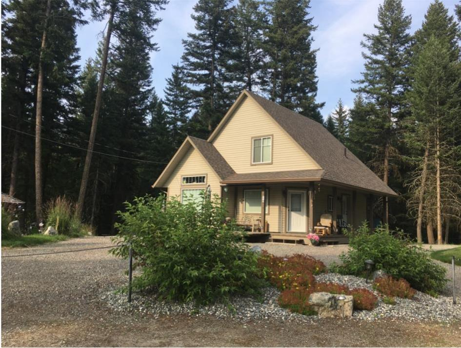
*Figure 14 This home demonstrates several FireSmart landscaping attributes. The gravel provides a non-combustible surface creating a break from direct flame contact to the home. Conifers have been removed up to 10m away and ladder fuels have been cleared. Leafy, deciduous plants are the preferred vegetation to be found in zone 1.*
