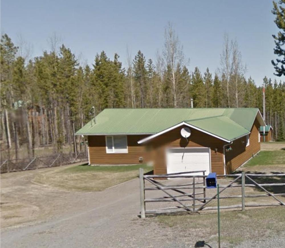
*Figure 8 The presence of nearby combustible debris (such as wood pallets, ladders, building materials etc.) and combustible plants pose a high risk to ignition of a building's exterior. In Lac Le Jeune, many homes were seen free and clear of debris and plants within the non-combustible zone (0-1.5m from furthest extent of home).*
