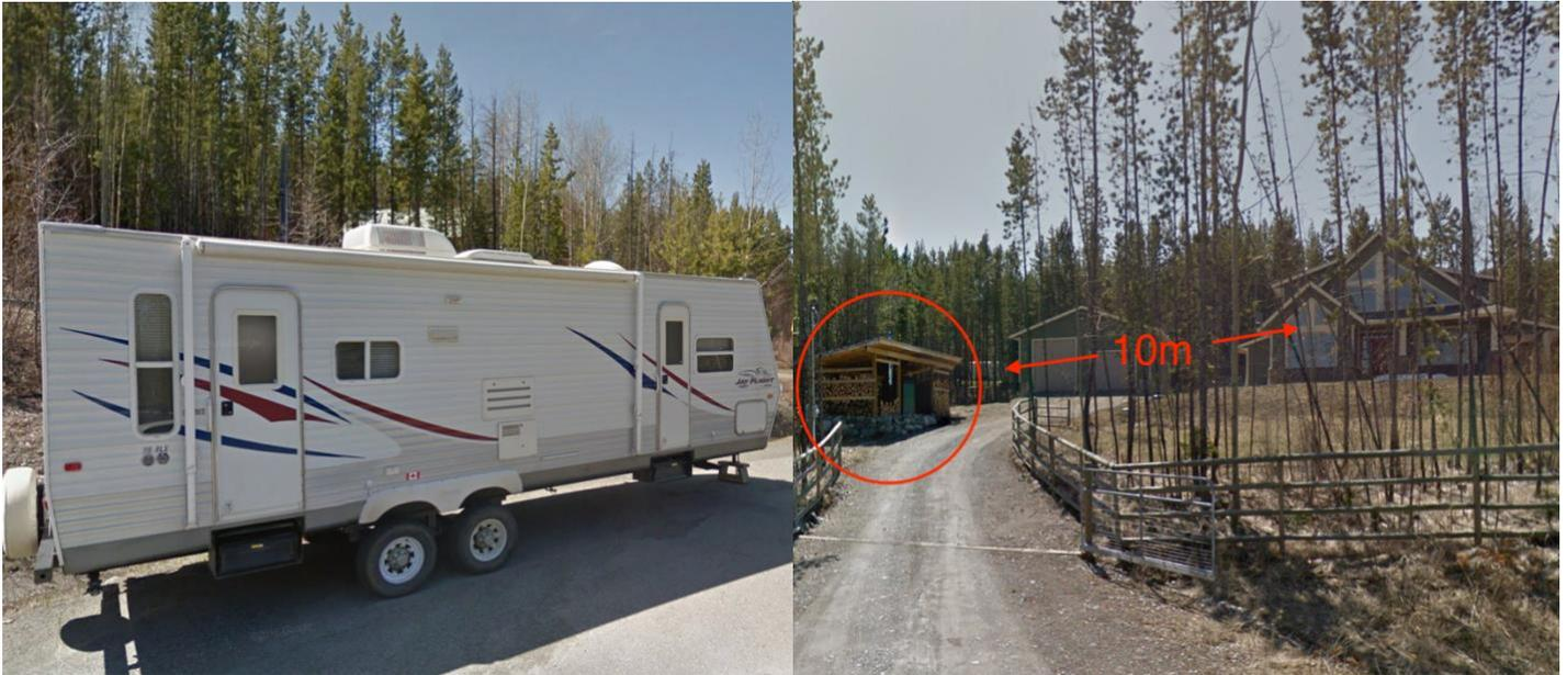
Figure 9 Combustibles such as firewood and other personal items (i.e. campers, trailers, RVs, etc.) should be stored 10m away from the home
