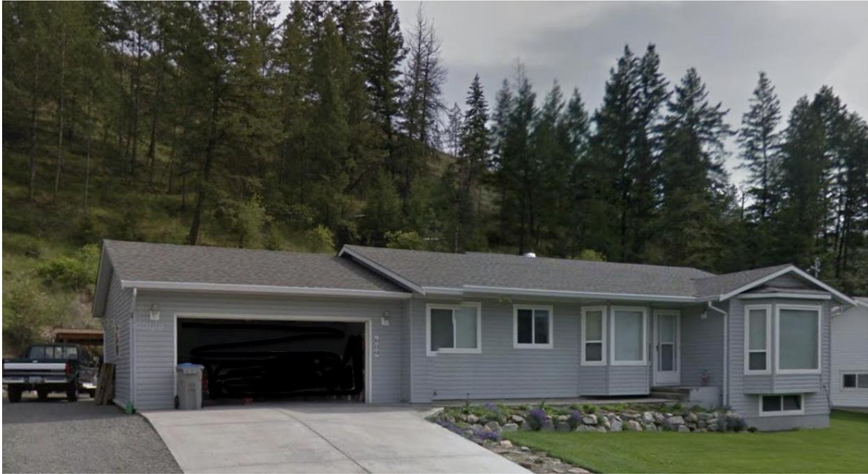
*Figure 13 Concrete driveway, walkway and gravel help to disconnect the home from potential direct flame contact. Grass is kept green and at low growth therefore reducing the likelihood of intense burning. All other vegetation is kept 10m away from the structure.*
