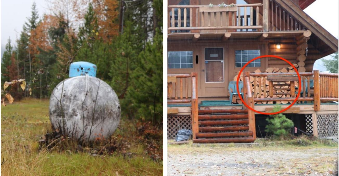
*Figure 9 Both propane and firewood pose significant risk to home ignition during wildfire event when they're found within 10m of a home. As well, they're more likely to ignite when in contact with vegetation. By establishing fuel free zones homeowners can mitigate this risk.*
