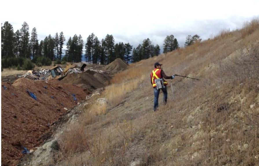
**Photo 1. SHA Staff conducting baseline methane emission sampling at Heffley Creek Landfill**
