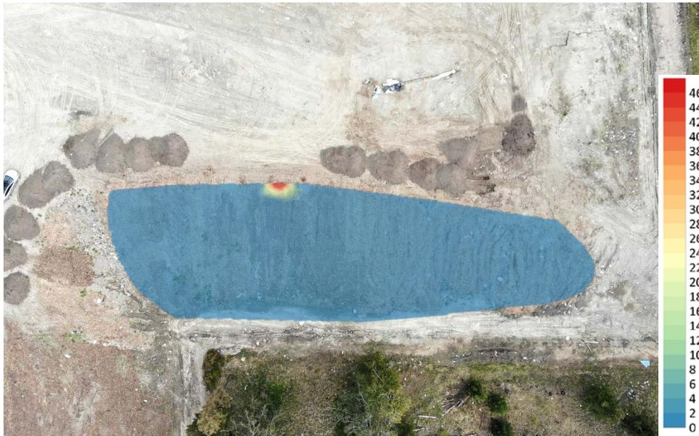
**Photo 8. Surface Methane Concentration (ppmv) and Methane Emission Hot Spot in S5 Area**
