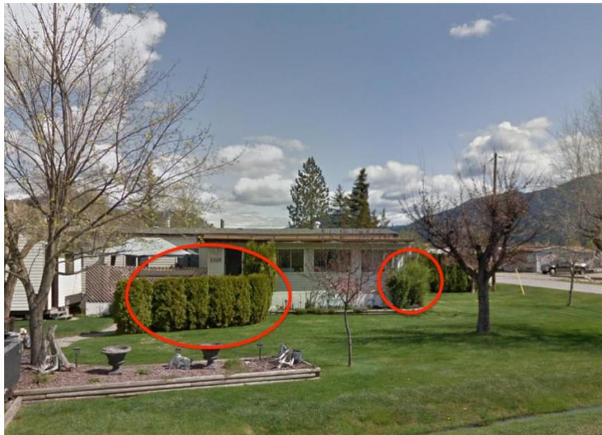
*Figure 8 The presence of nearby combustible debris (such as wood pallets, ladders, building materials etc.) and combustible plants pose a high risk to ignition of a building's exterior.*
