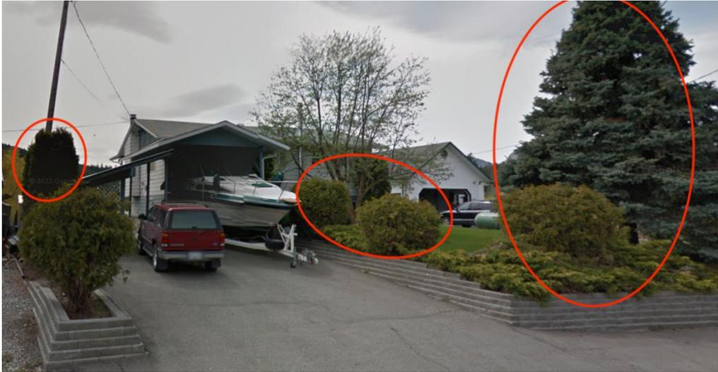
Figure 12 Combustible plants, including conifer tree species, should be removed from Zone 1 (0-10m)
