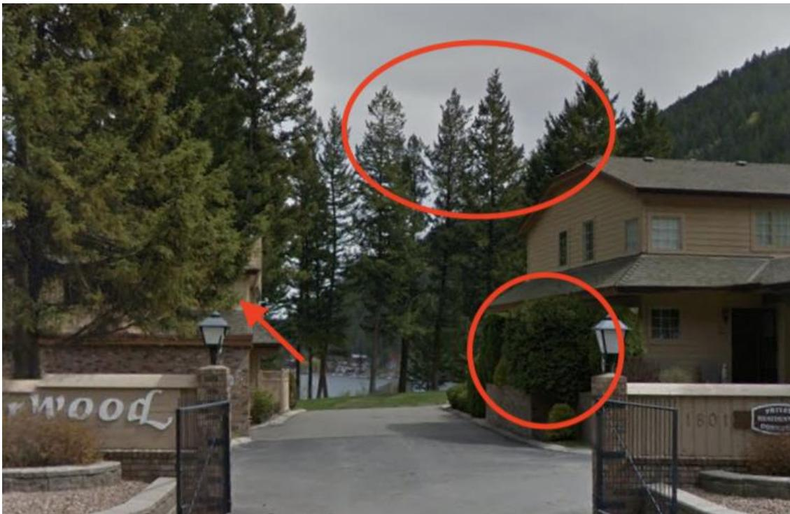
*Figure 7 Juniper and Cedar shrubs and hedges within Zone 1a (0-1.5m) and conifers – Douglas fir – located in Zone 1 (1.5-10m) pose an increased risk to home ignition due to the ability of easy ignition and ability to sustain high-intense heat.*
