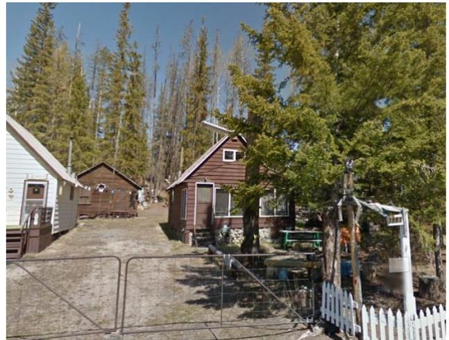
*Figure 10 Conifers within 10m of the home pose a significant risk towards home ignition. This is due to the relative ease of ignition and ease of fire transference from the ground to aerial fuels, creating increased fire intensities.*
