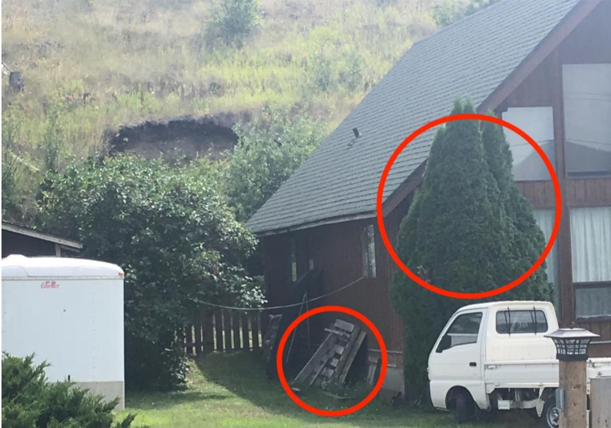
*Figure 8 The presence of nearby combustible debris (such as wood pallets, ladders, building materials etc.) and combustible plants pose a high risk to ignition of a building's exterior. (photo not taken from Iron Mountain)*
