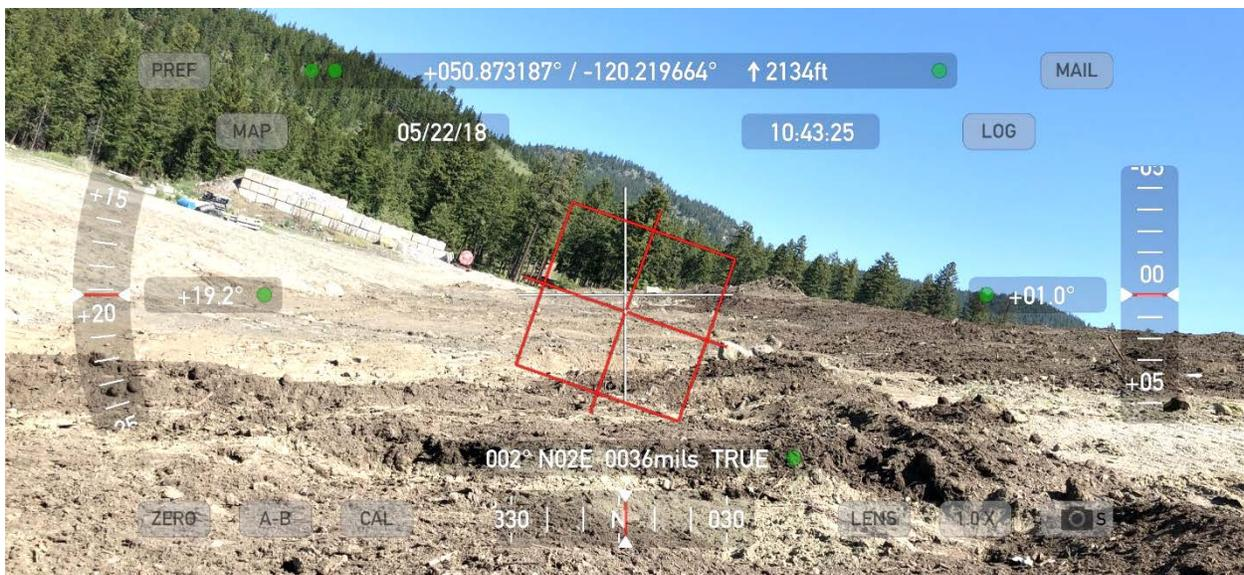
**Photo 4. Proper side slope in Area Slope 4 (3H:1V)**
