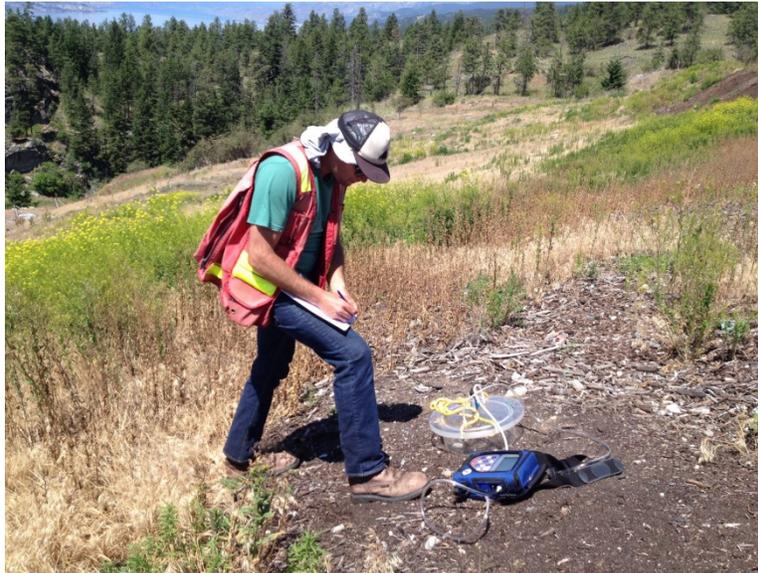
**Photo 5. Methane Emission Measurement Using Flux Chamber**
