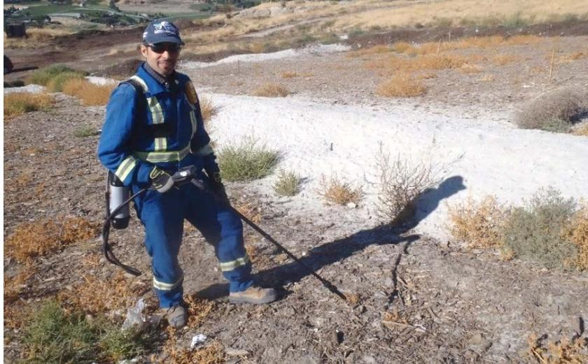
**Photo 6. Surface Methane Concentration Scan Using a Portable FID Instrument**
