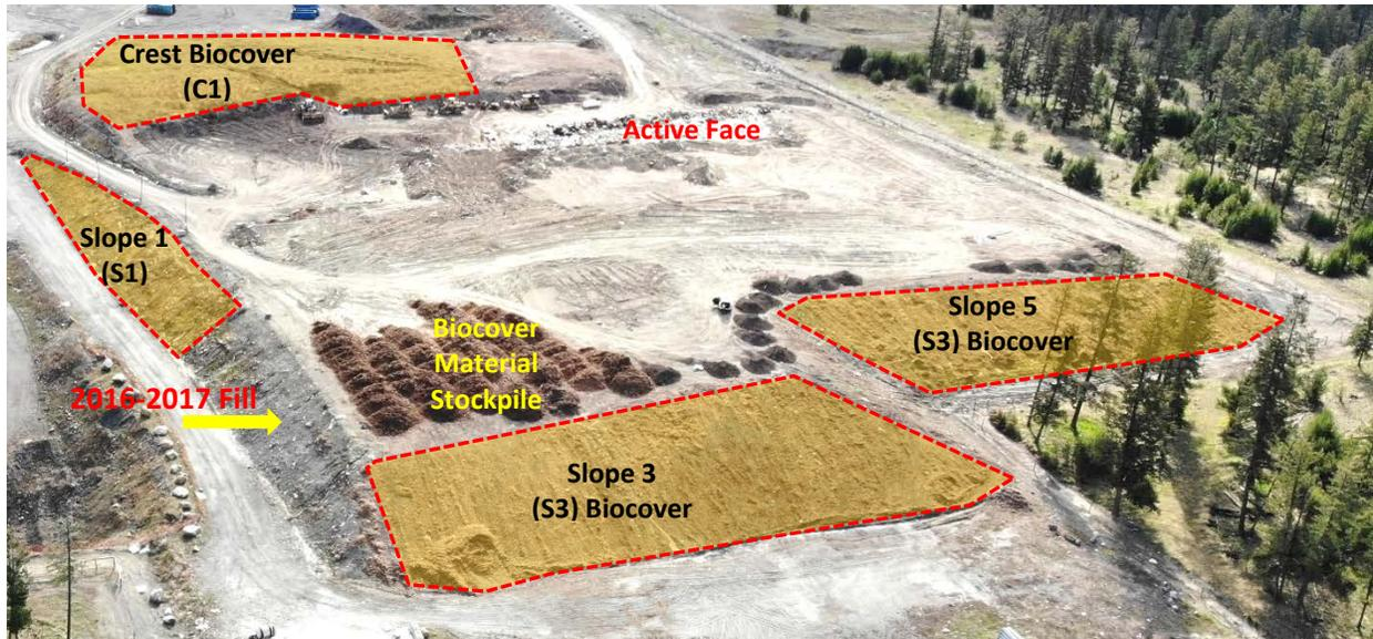
**Figure 3. Slope 1 (S1), S3 and S4 Biocover Areas at the Heffley Creek Landfill**
