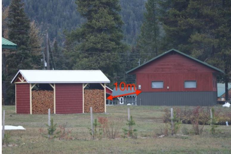
*Figure 10 this home is a good example of FireSmart storage of firewood. The firewood is located 10m away from the home and has been provided some protection from embers. Removing any continuity of vegetation (i.e. remove a perimeter of grass) would help to further decrease the likelihood of ignition.*
