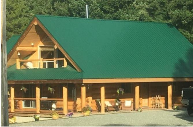
*Figure 11 Fire-resistant roofing material provides excellent resiliency against home ignition. Simple roof designs can also contribute to the reduction of debris accumulation as pinch points are no longer a factor*
